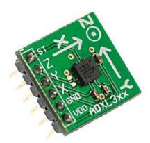
Fig. 3: ADXL355 accelerometer sensor
