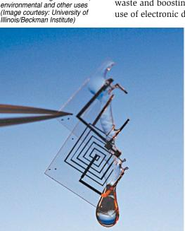
lectronic devices are built to last. But now their lifespans can be con-**⁴**trolled, courtesy burgeoning research into transient electronics, or devices that are meant to serve a specific function before completely dissolving into their environment over a predetermined span of weeks, months or even years. Moreover, with a degrading environment where electronic waste also plays a major role, the need for such electronic devices that can be disposed of when we want increases.
